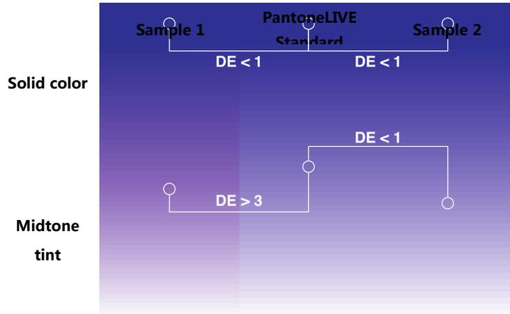
**Figure 2: Tint variation of an in-tolerance solid color**
